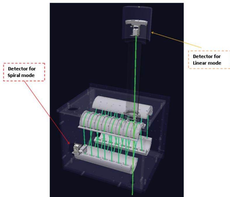
Figure 2. Ion trajectories of the JMS-S3000 SpiralTOF™.
