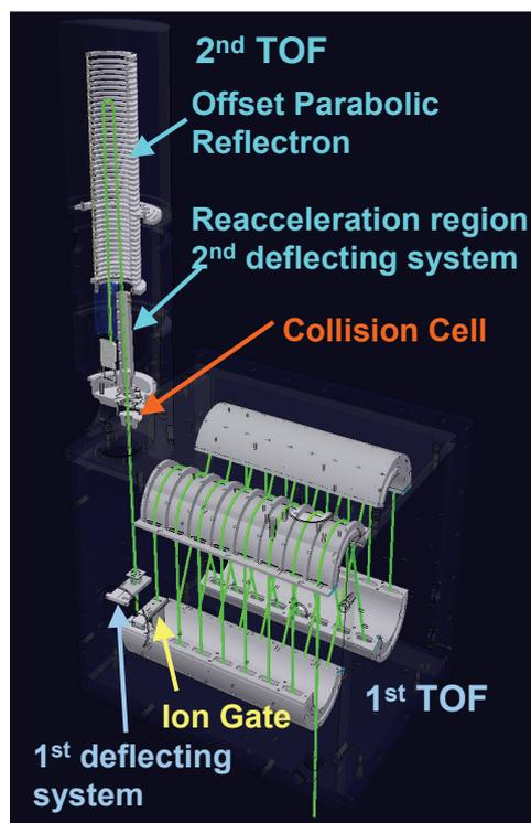
Figure 2. Ion trajectory of SpiralTOF and TOF-TOF attachment.
