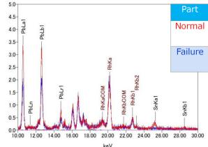
B) Failure part (crack)
